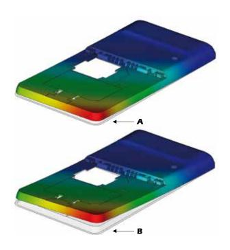
The Moldflow analysis clearly shows the difference in warpage between Grivory GVX (A) and conventional products with the same amount of glass-fibre reinforcement (B). This reduced warpage is not only Moldflow-Theory. Both test bars and daily applications confirm this lower warpage in an impressive manner.
