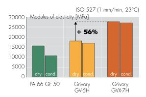
Grivory GVX achieves modulus of elasticity values of nearly 30'000 MPa. Compared to values for Grivory GV, this is an increase of more than 50%! These values also remain at the highest level for test bars in a conditioned state where conventional polyamides show a decrease of up to 35%.
