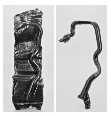
Fig. 14: Blow moulding produced by the conventional process (left) and 3D blow moulding (right).
